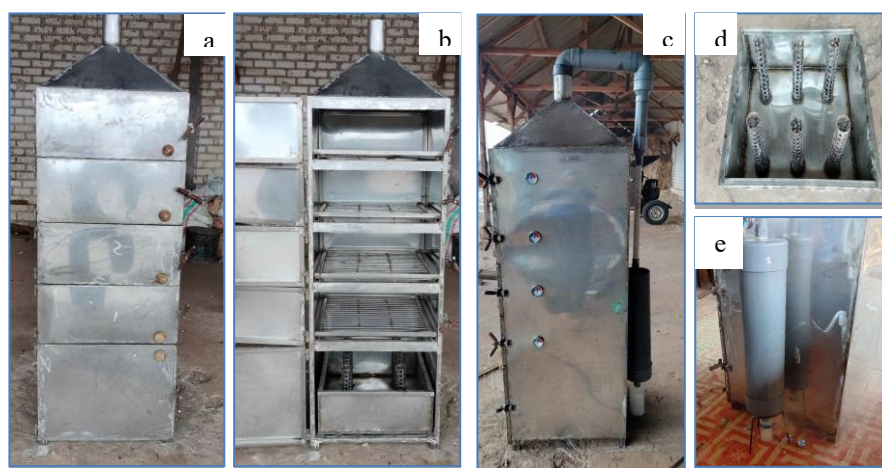
Fig 1. The Modified Efhilink Smoking Cabinet (a) front view, (b) stacking rack model, (c) side view, (d) rack for burning materials, (e) pyrolysis technology producing liquid smoke
