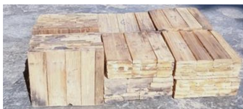
Fig 2. Model (a) zig zag , (b) parallel Laminated
