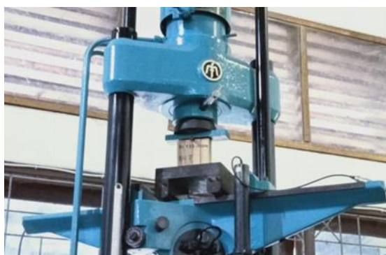
Fig 1. Strength Testing of Bamboo Buds Laminated
