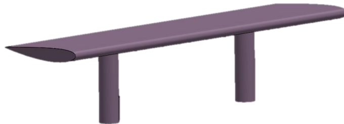
Fig 5. Aerodynamic Profile 2414 was modeled in 3D, and supports were considered for structural analysis evaluation
