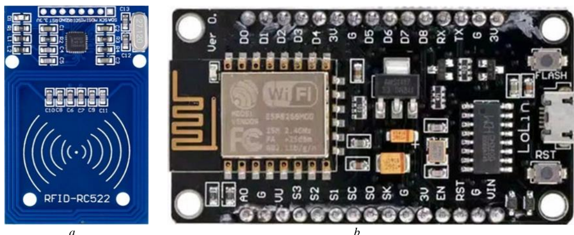
Fig 2. Hardware: a – MFRC-522 Module; b NodeMCU ESP8266 microcontroller
